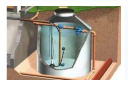
80% of the average intensity of rainfall in Germany is under 15 I/(sxha), resulting a volume flow rate of 0.32 I/s with a roof area of 213 m<sup>2</sup>.
